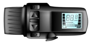
The operation of the Mini LCD system has four selectable POWER levels. Level 1 gives 25% of the power, level 2 - 50% up to level 4, 100% power. Speed range is from 0 to 15 mph in all levels. This is available as an easy to fit upgrade.
